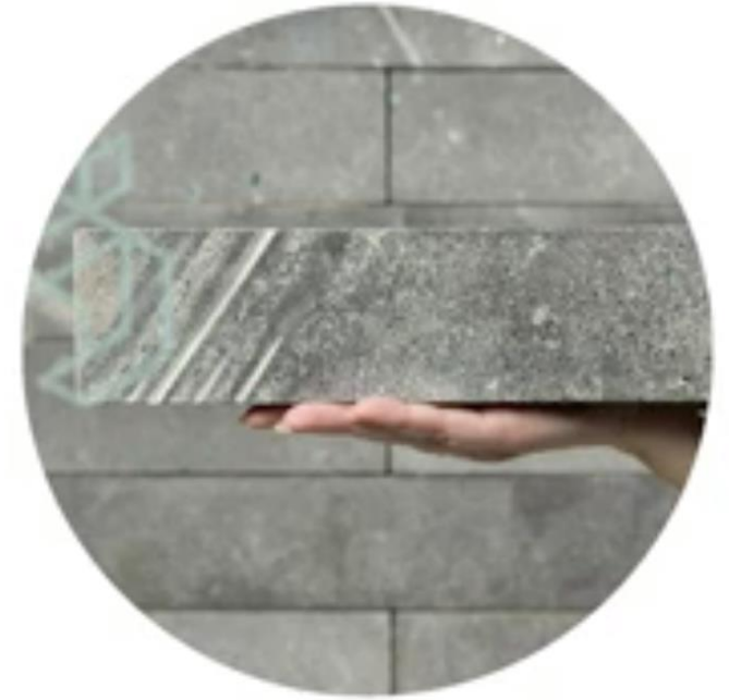
Creating Bricks at Room Temperature Using Grey Water
